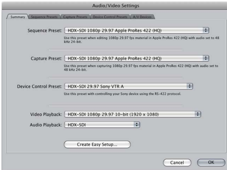
Figure 7-2: HDX-SDI Easy Setup settings can be adjusted in Final Cut Pro's Audio/Video Settings window.
