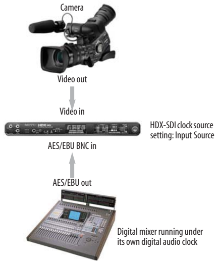
Figure 3-14: Capturing digital audio from a device that is not resolved with the HDX-SDI. In this case, sample rate conversion is used.
