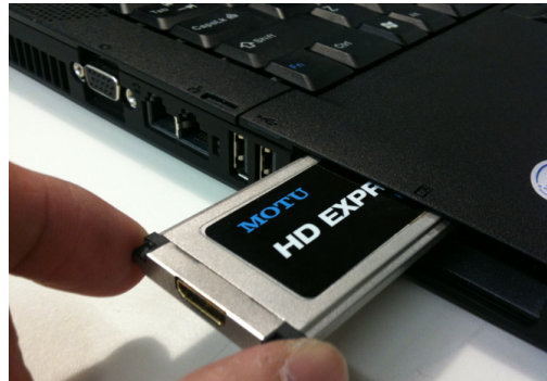
Figure 4-2: Inserting the HDX-SDI ExpressCard adapter.
