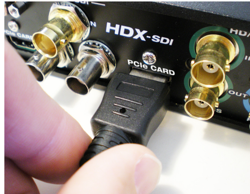
Figure 4-4: Making the connection from the computer to the HDX-SDI.
