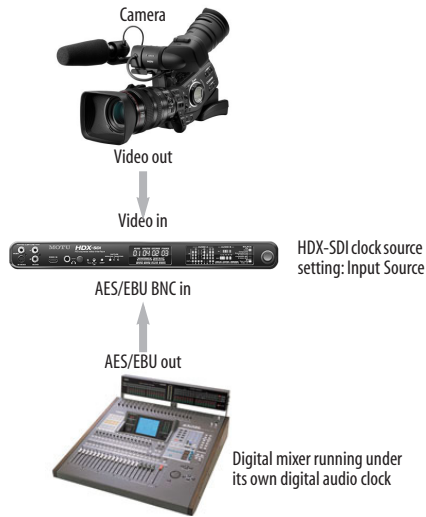
Figure 4-16: Capturing digital audio from a device that is not resolved with the HDX-SDI. In this case, sample rate conversion is used.
