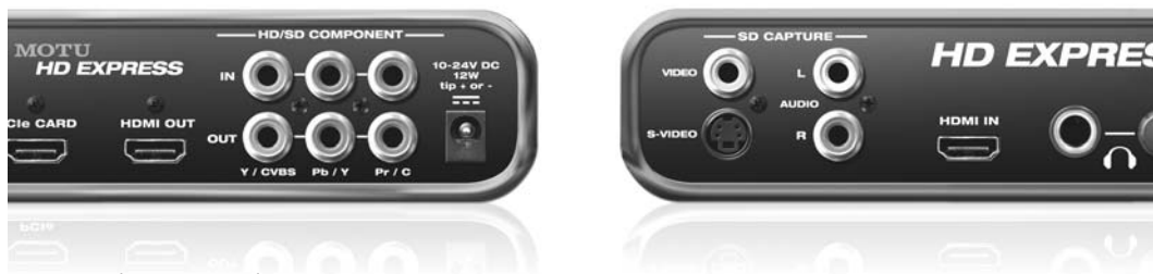
Figure 3-3: The HD Express video connectors.
