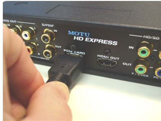
Figure 3-2: Making the connection from the computer to the HD Express.
