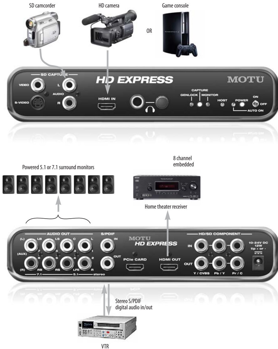
Figure 3-6: HD Express audio connections.
