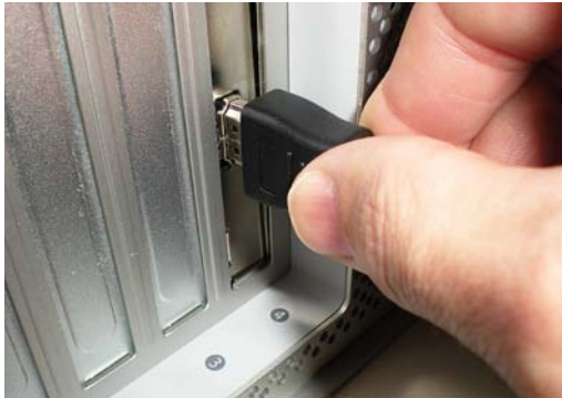
Figure 3-1: Connecting the HD Express to the computer.
